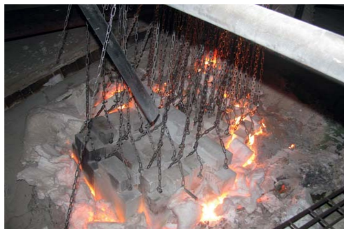
View outside after insert of suspension bricks 悬吊砖放入后外部
